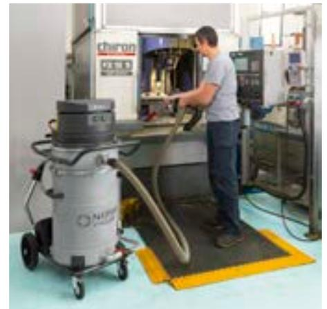
*Recovery of chips and oil from a machine tool.*
