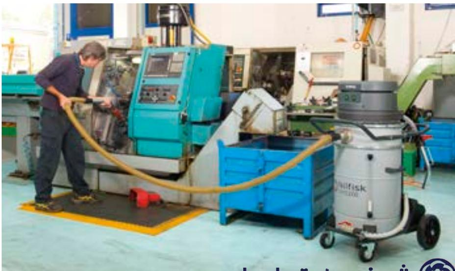
Collection of chips and coolant from a machine tool
