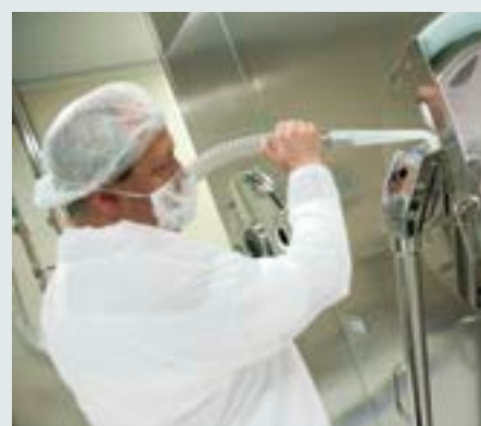
Cleaning of a coating pan
