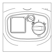
The motor speed and the suction power can be varied with the suction power control. This allows precise adaptation of the suction power for different cleaning tasks.
