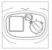
Before switching the switch to position "auto", ensure that the tool connected to the appliance socket is switched off.
