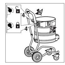
be reduced. Before reinserting the suction hose: clean the inlet fitting and hose collar.
