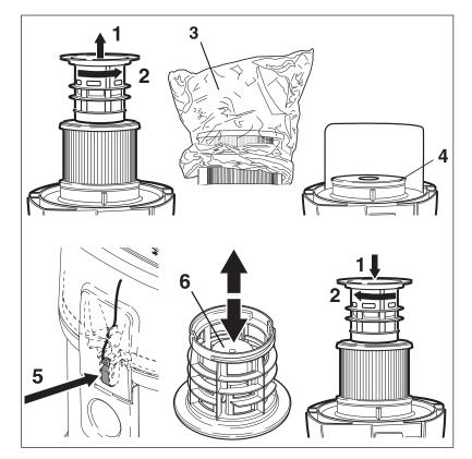
7.2.6 Replacing filter element (IVB 5-M/7-M)
