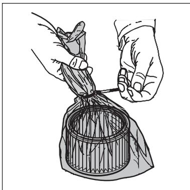
8. Carefully remove the filter element and close the protective filter bag with a knot.
