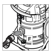
10.Connect suction hose to inlet fitting "H" (down) (F).
