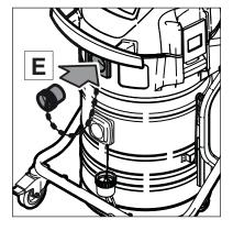
9. Close "M" inlet fitting (top) with plug (E).
