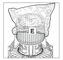
7. Place the protective filter bag over the filter element.
