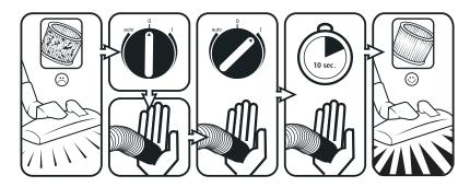
To ensure that suction performance is always at its best, the filter element is automatically cleaned during operation. We recommend complete cleaning if the filter element becomes extremely dirty.
