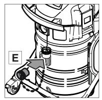
9. Close inlet fitting "H" (down) with plug (E).
