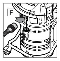
10.Connect suction hose to inlet fitting "M" (top) (F).
