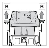
Open the retaining clamps (B) and remove the upper section of the vacuum cleaner.
