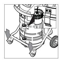
Check the antistatic clamps for damage and have them replaced by Nilfisk-Advance Service if necessary.
