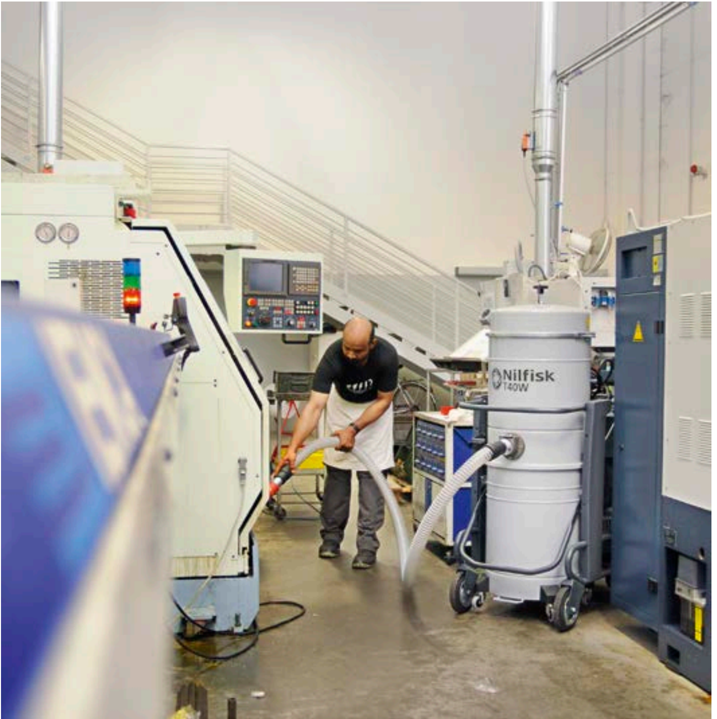
Recovery of oil and shavings.
